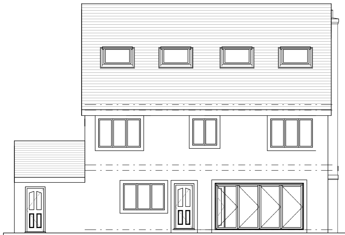
Proposed Rear Elevation 1 : 100
